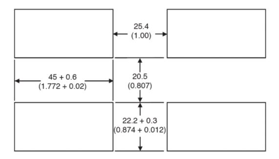
From the front of the panel, slide the housing through the cutout. The housing gasket should be flat against the housing flange before installing.
